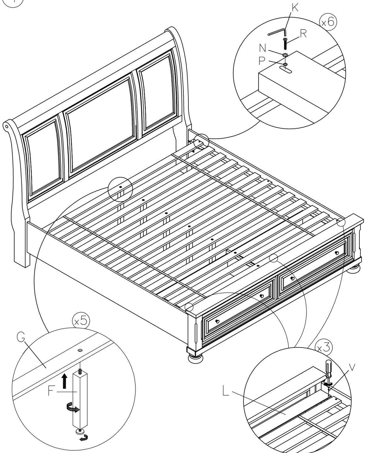
Turn Adjustable Leveler on the bottom of the Cross Slat Center Leg F until it contacts the floor.
